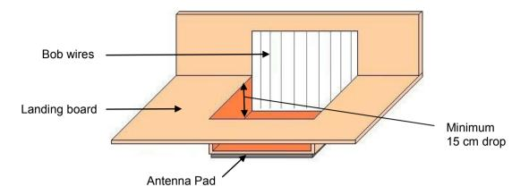
On the landing board, you should build an area which is lower, under which the antenna pad is then installed. The pigeons will then step onto the antenna pad one by one and not all at the same time and as a result the registration of the birds is optimised.
