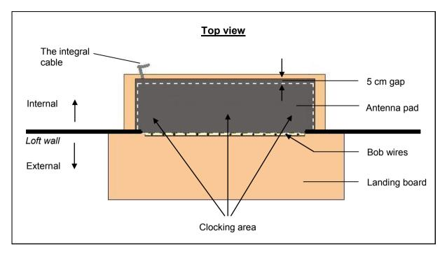
Antenna pad positioned inside of the loft entrance and behind the bob wire
