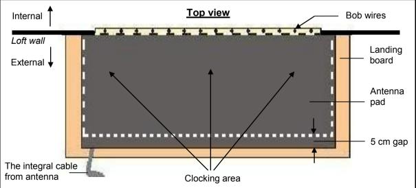
In this set-up, install the antenna pad with the integral cable leading to the <u>outside</u> of the loft.
